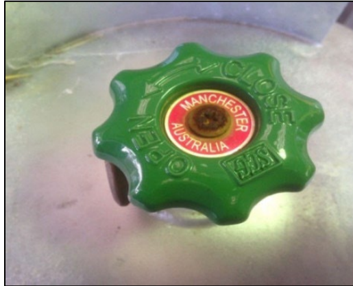
Figure 20. Exchangeable gas cylinder showing green tap with 'OPEN' and 'CLOSE' markings
