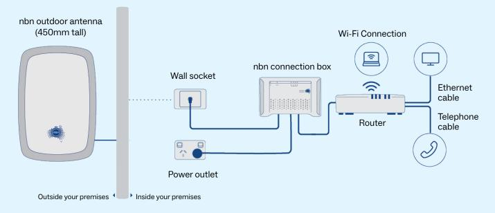
The nbn outdoor antenna is attached to the outside of a premises, in a location that provides direct line of sight to an nbn Fixed Wireless tower. A cable is then used to connect the outdoor antenna to the nbn connection box inside.
