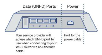
The nbn connection box is wall-mounted and has four Ethernet ports that can deliver internet data. It requires power to operate and can only be installed by an nbn approved technician.
