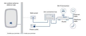
End users can connect their devices directly to the nbn connection box via an Ethernet cable. If they prefer to connect via Wi-Fi, they'll need to connect their own router, or one supplied by their Retail Service Provider, to the nbn connection box.
